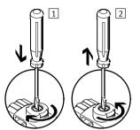
1 Press in the stem of the MO with a pin or screwdriver until the valve switches and then turn the stem clockwise by 90° until the stop is reached.
