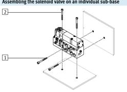
Assembling the solenoid valve on an individual sub-base
