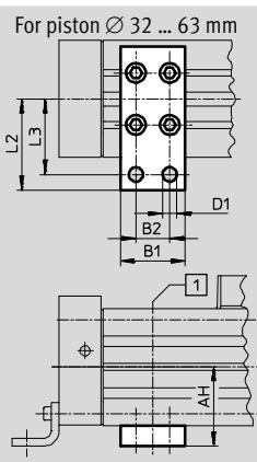
**[1]** Position of the central support along the profile barrel is freely selectable.
