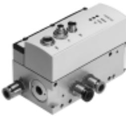
The 5/3-way proportional directional control valve for applications with Soft Stop and pneumatic positioning. Fully digitalised – with integrated pressure sensors, with new diagnostic functions. In sizes 4, 6, 8 and 10. Flow rate of 350, 700, 1400 and 2000 l/min.
