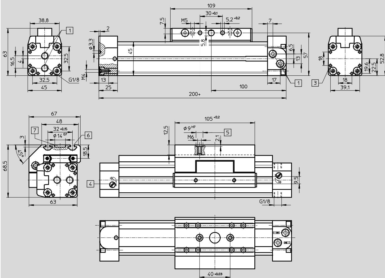
[1] Supply port at one end, optionally on three sides of an end cap (D2 variant: supply port at both ends, optionally on three sides per end cap)
